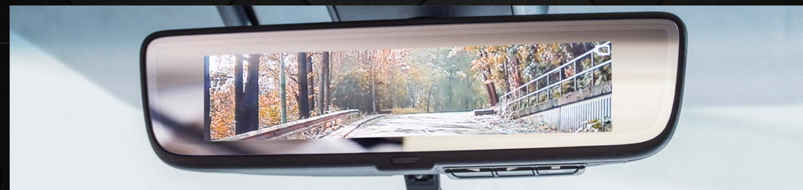
電子影像倒後鏡，清晰顯示車後路面情況 Digital Inner Rear-view Mirror shows the road conditions behind the vehicle
