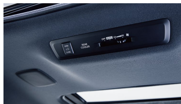
中後排冷氣系統控制及出風口 Rear Air-conditioning System Control Switch and Register
