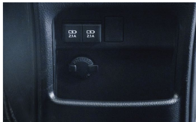
USB 插座及 DC 12V 電源插座 USB charging Ports and DC 12V Power Outlet
