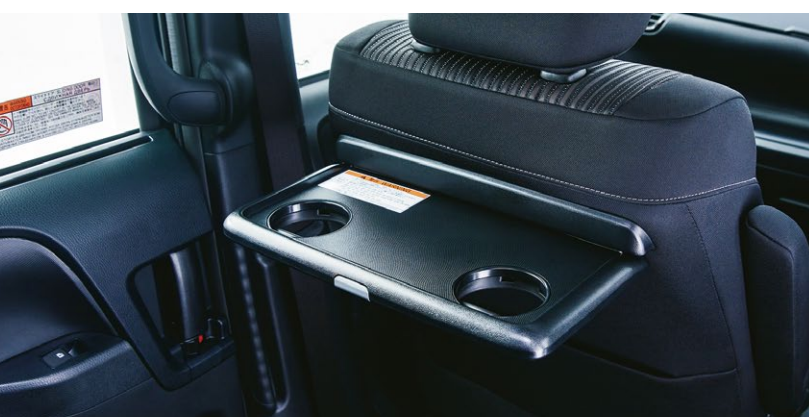
前排乘客椅背新設摺合式檯面，收放自如 Front Passenger Seat Back with Retractable Table
