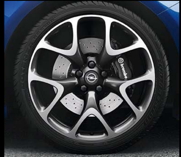
Alloy wheel. 8.5 J x 20", OPC, weight-optimised, tyres 245/35 R 20 (R01, optional).
