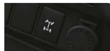
Rear Differential Lock System The system helps secure traction when driving in muddy terrain or in the unlikely situation when the vehicle is stuck. (All Type Double Cabin; Single Cabin DSL 4x4 Type)
