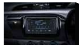
New Flat Head Unit Design Equipped with capacitive screen which can be connected to Radio, USB, AUX, Bluetooth* for entertainment on the go. (G & E Type Double Cabin) * Bluetooth only available on G Type.
