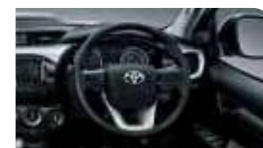
Steering Switch (Audio, Telephone, VR, MID) Steering wheel designed for excellent operability, incorporating control switches for audio, telephone, VR and MID. (V & G Type Double Cabin)
