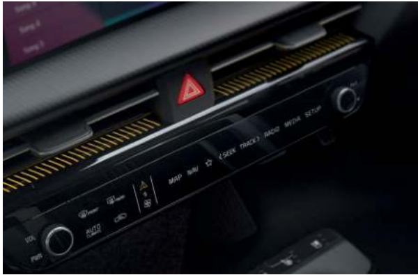
Infotainment/climate switchable controller. The switchable controller offers an intuitive way to interact with the car, while keeping all important information easily accessible. Press the one-touch infotainment icon or climate icon, and the relevant menus to make any adjustment you desire.
