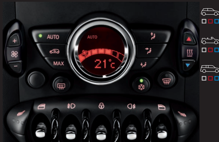
2. Automatic air conditioning
