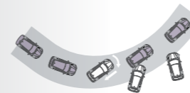
Lateral Rear-Wheel Slippage Braking force is applied to the outer front wheel to prevent spin-out.
