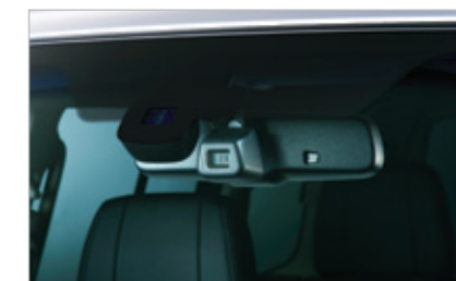
Auto Dimming Rearview Mirror & Rain Sensor (Executive model only)
