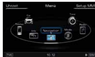
Menu: Display of the 7 available submenus which can also be alternatively selected using the hard keys.
