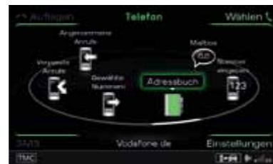
Phone: The available mobile phone Bluetooth interface has a selection screen containing call lists, directory and selection interface as the start-up setting.
