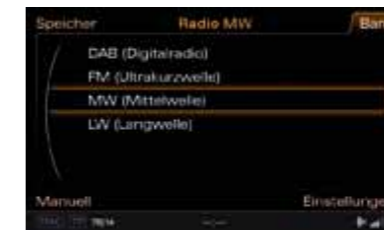
Radio: The integral radio receiver is set up for VHF, LW and MW radio with a continually updated station list.
