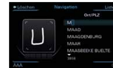
MMI touch: You can "write" on the MMI® touch using your finger. The system recognises letters and numbers. Compatible with the telephone; additionally you can thumb through the albums of your music collection in the jukebox with a brief stroke of the finger.
