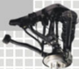
Rear multi-link suspension
