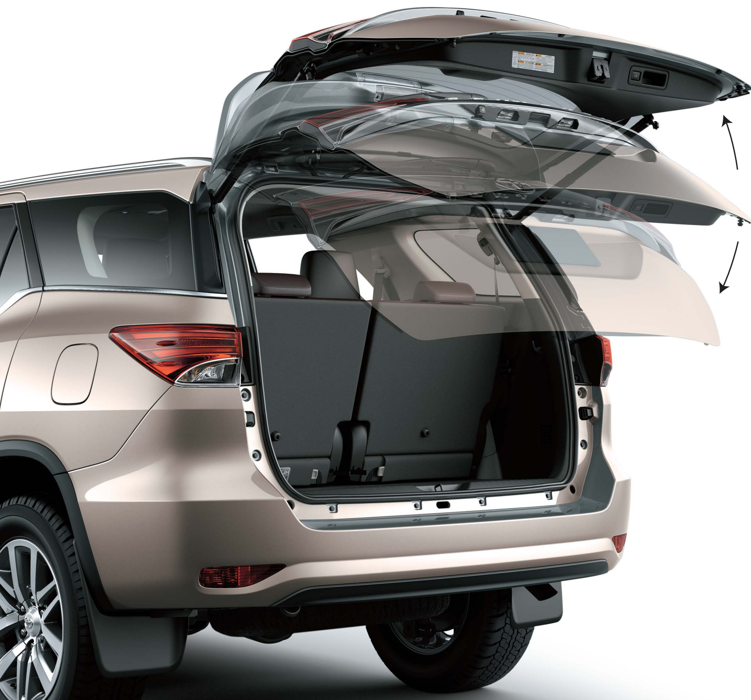
Electronically Controlled Power Back Door with Memory and Jam-Protection
