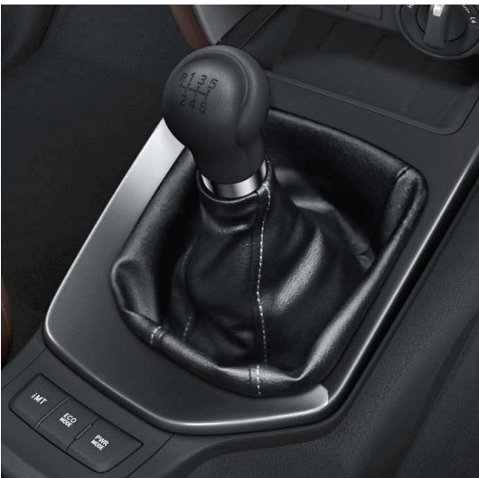
6-Speed Intelligent Manual Transmission (iMT)
