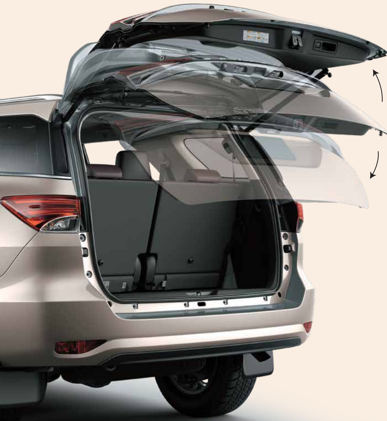
Electronically Controlled Power Back Door with Memory and Jam-Protection
