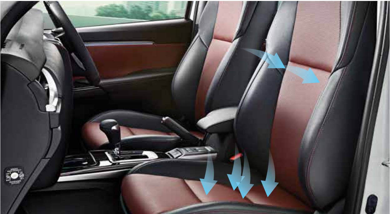
Superior Suction based Seat Ventilation System
