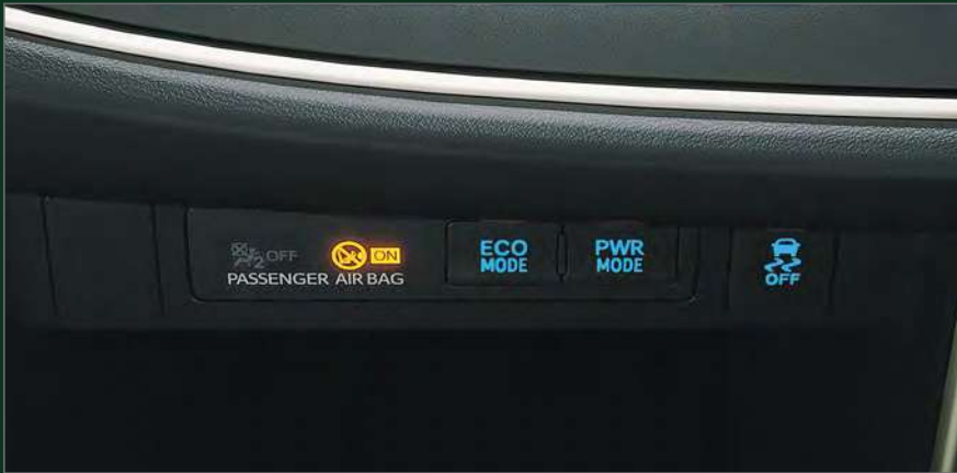
ECO & POWER Drive Modes to choose between 2 distinct driving modes. ECO mode for optimum fuel economy and POWER mode for sharper acceleration response
