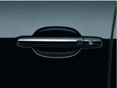
The “keyless access” locking and starting system: When the door handle is touched, the electronics of the vehicle communicate with the key. The doors are unlocked and the Memory package activated even if the key is in your pocket.
