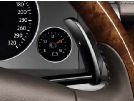
Tiptronic operation: Formula 1 style gear-changing in the Phaeton with the steering wheel paddles facilitate ergonomic, sporty operation of Tiptronic.
