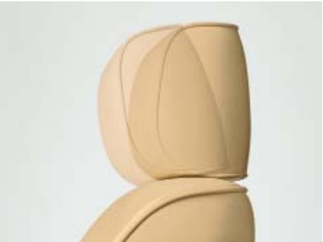
Safety for the spine: Active head restraints lessen the risk of whiplash injuries.
