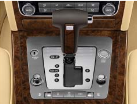
“Keyless access”: With the “keyless access” function the Phaeton can be started via the starter button without a key in the ignition lock.
