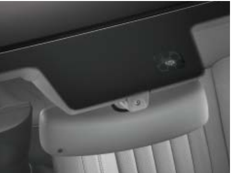
Safety in rain: The rain sensor automatically adjusts the speed of the windscreen wipers to the intensity of rainfall.
