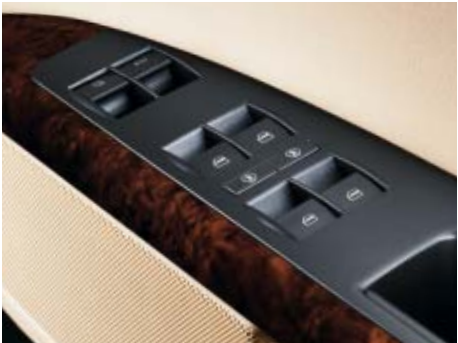
Control unit in the door: This operates many functions – from the electric windows to the fuel flap release.
