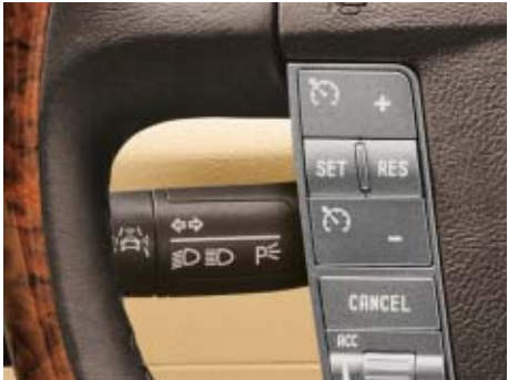
Cruise control: 30 kmph onwards, cruise control maintains the speed at the set level for additional comfort and convenience on long journeys in particular.
