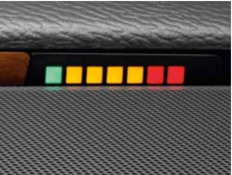
Park distance control: During parking and maneuvering, the system indicates how much space is left between the Phaeton and other vehicles or obstacles at front and rear. An acoustic and visual warning of the remaining distance is given inside the vehicle.
