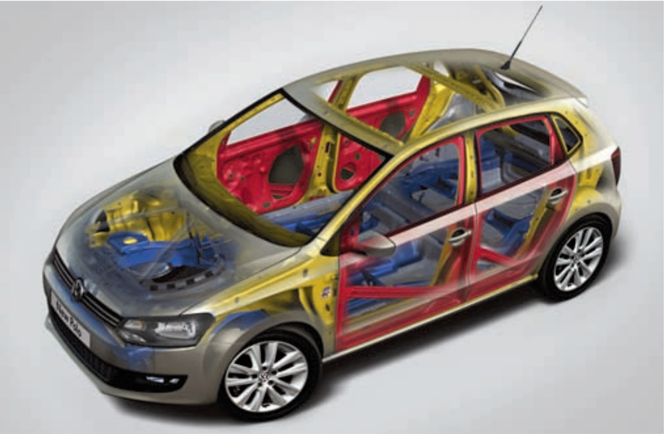
Passive safety: The Polo's high-strength steel frame makes it a tough car. This creates an indigenously structured passenger cell for added passenger safety.
