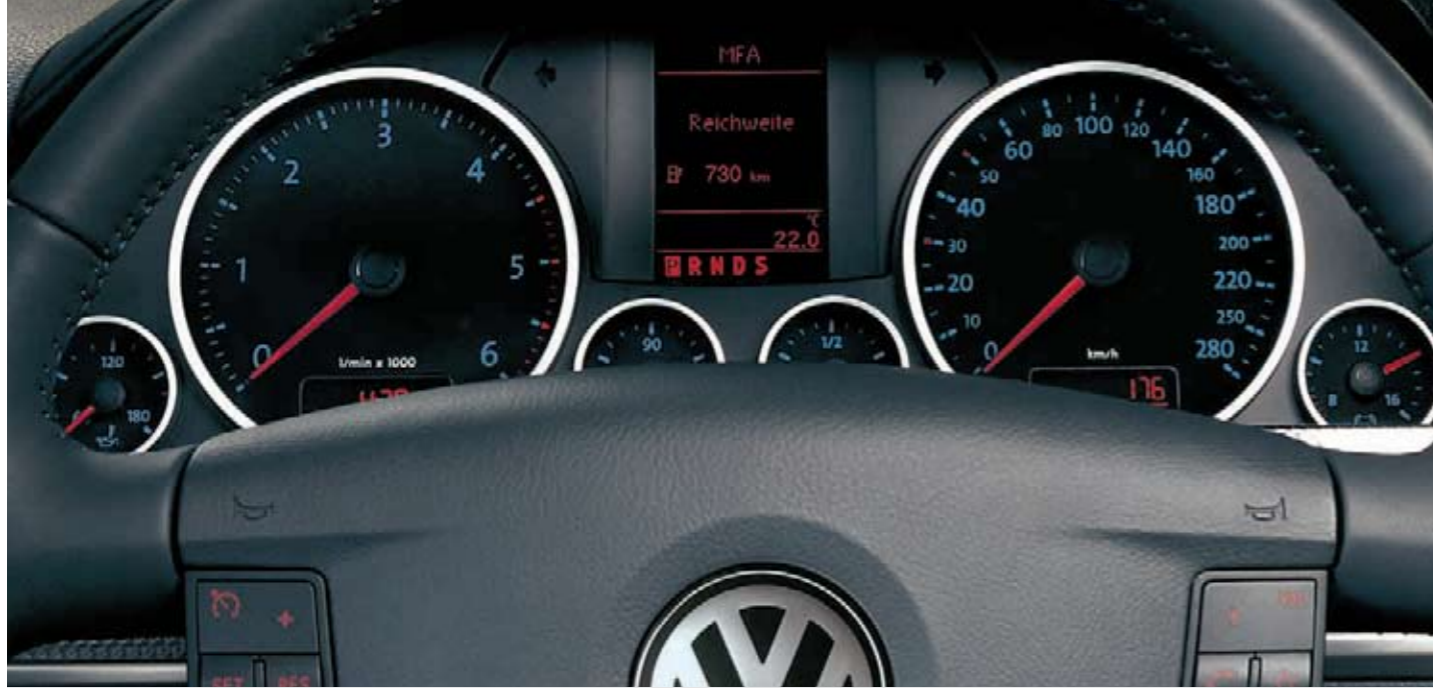
Multi-function two-colour display in the driver's field of vision shows, for example, the time, consumption and outside temperature.
