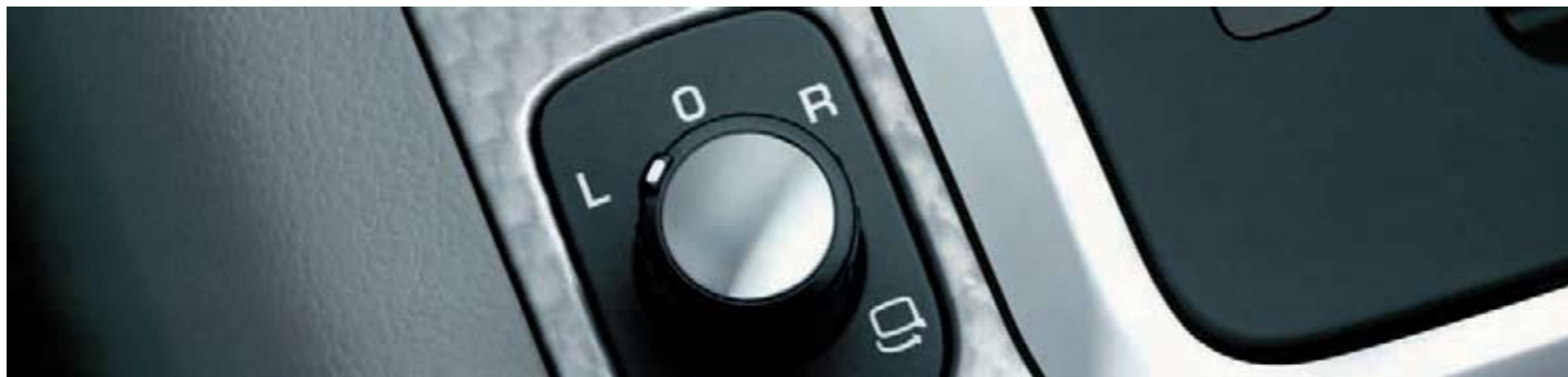
Control unit for electric door mirrors. Operates the adjustment, folding and heating functions.
