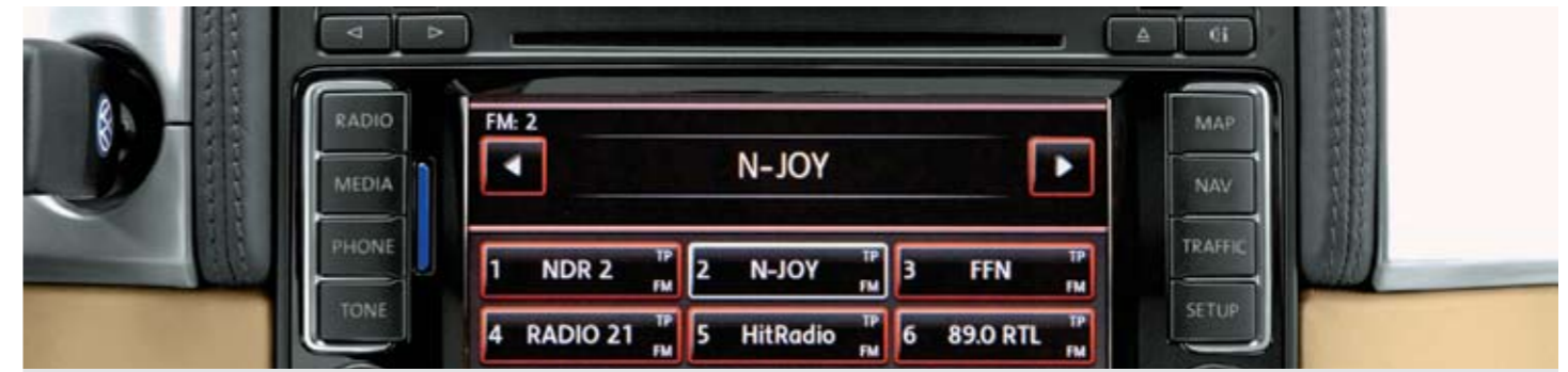
The audio module with ten loudspeakers and an output of 4 x 20 watts supplies perfect stereo sound at the front and rear. In addition to FM and AM radio reception, all common audio file formats such as CD, MP3 and WMA can be played.
