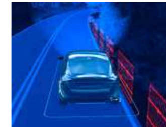
Run-off road Mitigation Our Run-off road Mitigation technology helps to keep you safe by keeping you on the road. If this innovation detects you are about to leave the road unintentionally at any speed between 65-140km/h, it uses steering input and, if necessary, brake support to guide you back on track.
