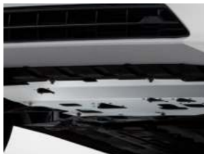
Protective Plate Beneath Engine.
