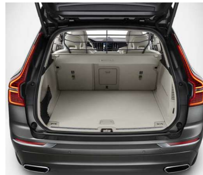
Protective steel grille.
