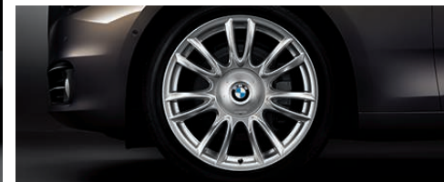
□ 20" BMW Individual light alloy wheels V-spoke 301 I with mixed tyres. Front: 8.5 J x 20 with 245/40 R 20 tyres. Rear: 10 J x 20 with 275/35 R 20 tyres.
