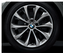
□ 19" light alloy wheels Turbine styling 452 with mixed tyres. Front: 8.5 J x 19 with 245/45 R 19 tyres. Rear: 9.5 J x 19 with 275/40 R 19 tyres.
