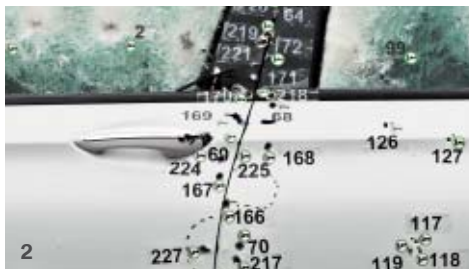
1. Special composite glazing for side windows and front windscreen, with a polycarbonate coating on the inside to prevent spalling. 2. Precisely fitted overlapping steel armour panels ensure integrity of joins. 3. Extensive ballistic testing with full metal jacket and armour-piercing, rigid core ammunition of various calibres.
