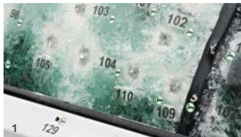
1. Special composite glazing for side windows and front windscreen, with a polycarbonate coating on the inside to prevent spalling. 2. Precisely fitted overlapping steel armour panels ensure integrity of joins. 3. Extensive ballistic testing with full metal jacket and armour-piercing, rigid core ammunition of various calibres.
