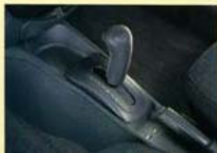
4-speed automatic transmission with 3 logic modes : sports, ice or normal
