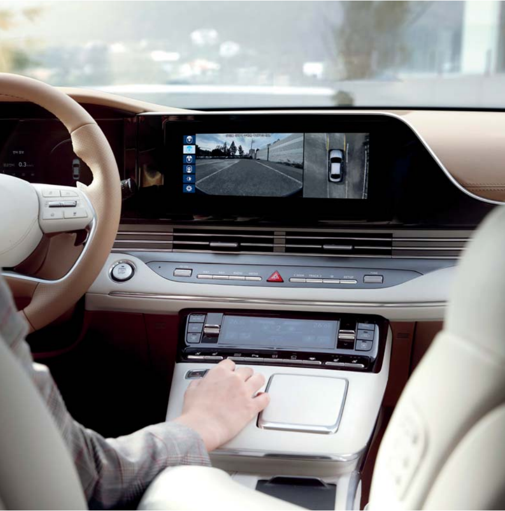
Surround View Monitor Four high-resolution cameras show blind spots in the front, rear, and sides so that the driver can park the car safely.
