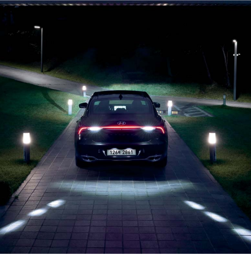
Back up guide light When the car is backing up, "guide lights" are projected onto the road behind the car to clearly show the driver's intention to back the car up to prevent accidents involving nearby vehicles or pedestrians.
