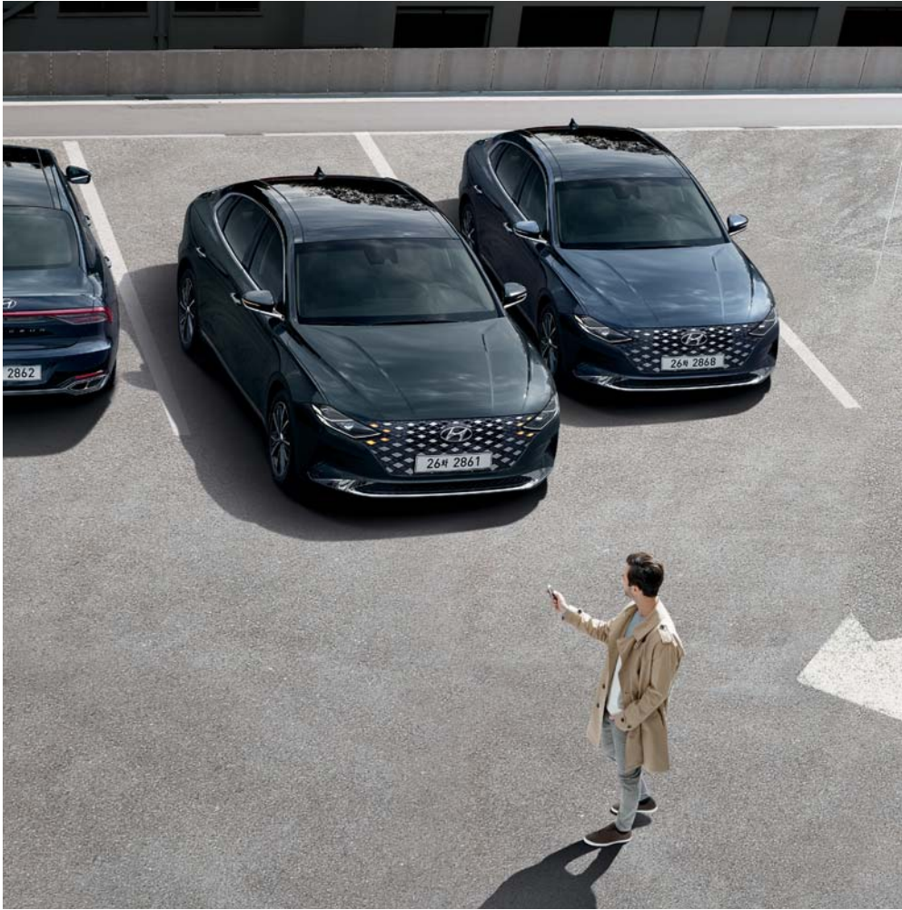
Remote Smart Parking Support Remote Smart Parking Support is a technology that helps the driver park, or passengers exit from, the vehicle in small, restrictive parking spaces. The smart key can be used from outside the vehicle to remotely control the vehicle and control backward or forward movement to ensure ease of parking.
