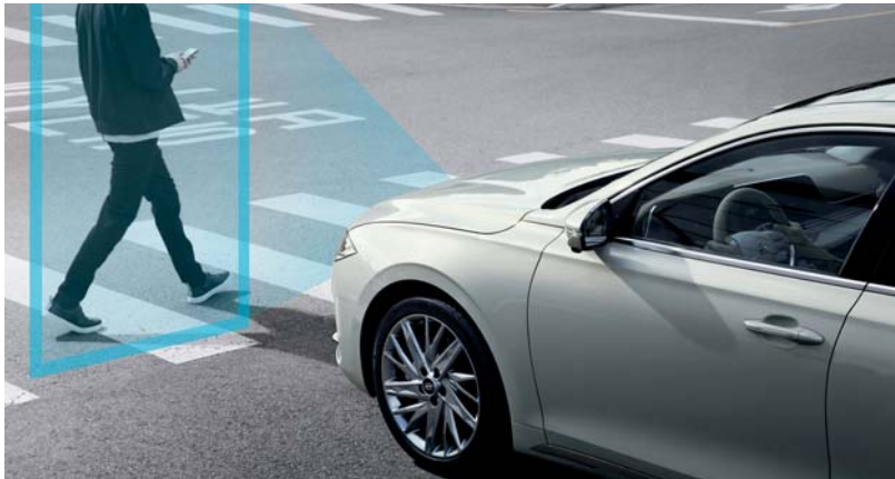
Safety Exit Assist If a vehicle is perceived to be approaching from the side or rear of the car after the driver has parked/ stopped, the child lock ensures that the rear doors remain locked. A warning is issued if all car doors are opened. Forward Collision-avoidance Assist After detecting a vehicle, pedestrian, or bicycle in front of the car (omnidirectional camera) or a car on the opposite side of an intersection and determining the risk of collision by analyzing the signals sent from the front camera and radar, the driver is notified of the potential risk with a warning. When necessary, the brake is activated to minimize damage.
