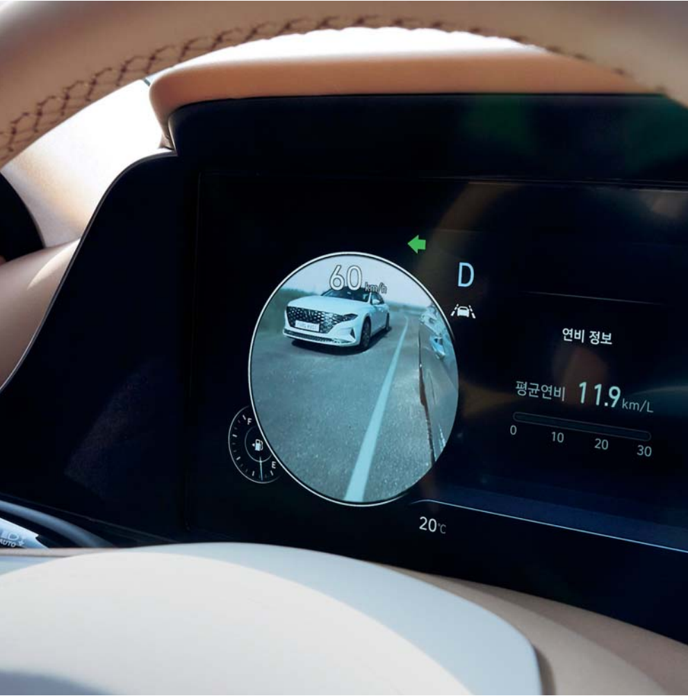
Blind-spot View Monitor When using the turn signal, the camera installed at the base of the exterior mirror displays videos of the left/right posterolateral views on the cluster screen. In the case the posterolateral view is restricted (driving in the rain, blind spots, etc.), the Sonata offers a clear and wide view to guarantee a safer driving experience.
