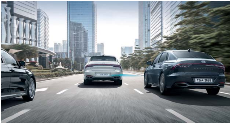
Highway Driving Assist Highway driving assist uses information, such as distance from the vehicle in front and road lane and navigational data, to control inter-vehicle distance and keep the vehicle inside the boundaries of the lane. It also minimizes driver fatigue during long-distance drives. Blind-spot Collision-avoidance Assist This function detects vehicles approaching from blind spots at the rear lateral end that are difficult to see in the exterior mirror, enhancing crash protection via warnings and brake controls.
