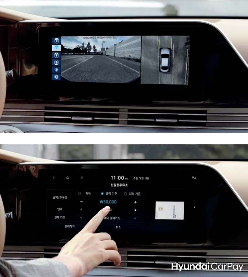
Surround View Monitor Four high-resolution cameras show blind spots in the front, rear, and sides so that the driver can park the car safely. It also offers enhanced convenience with the addition of three functions: front/rear top view, expanded top view, and reduced view.
