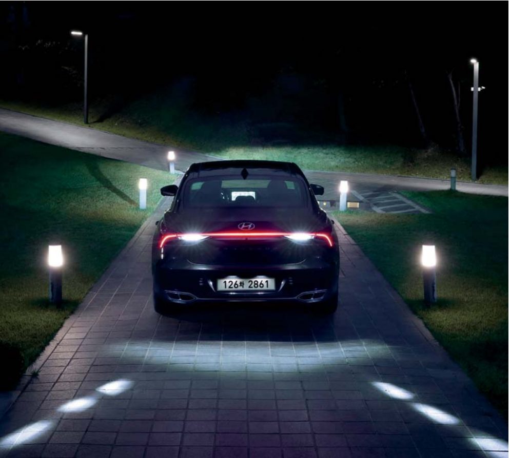
Back up guide light When the car is backing up, "guide lights" are projected onto the road behind the car to clearly show the driver's intention to back the car up to prevent accidents involving nearby vehicles or pedestrians.
