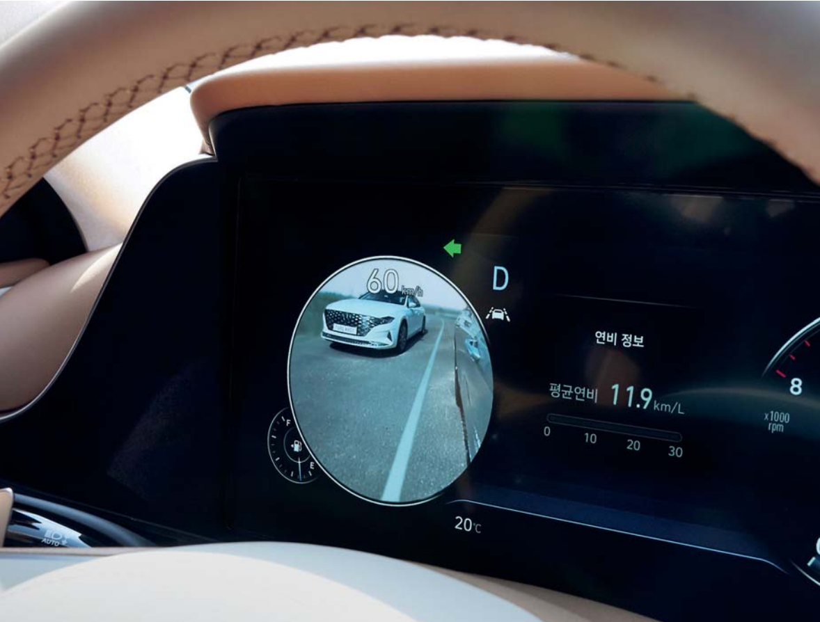
Blind-spot View Monitor When using the turn signal, the camera installed at the base of the exterior mirror displays videos of the left/right posterolateral views on the cluster screen. In the case the posterolateral view is restricted (driving in the rain, blind spots, etc.), the Sonata offers a clear and wide view to guarantee a safer driving experience.
