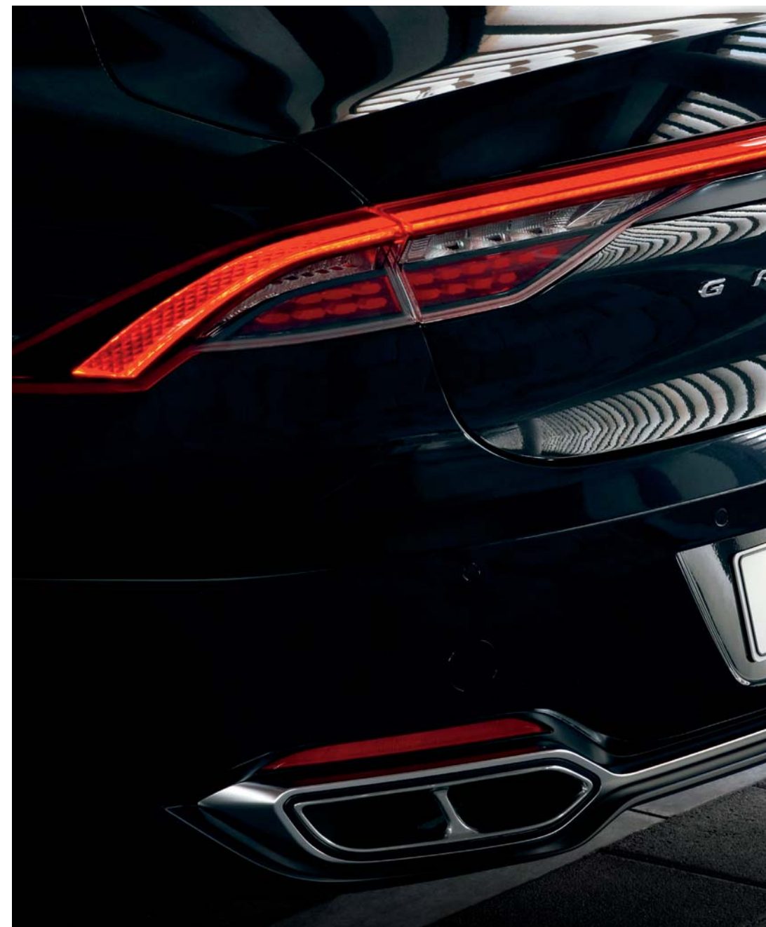
LED rear combination lamp (brake light, tail light and turn signal lamp)
