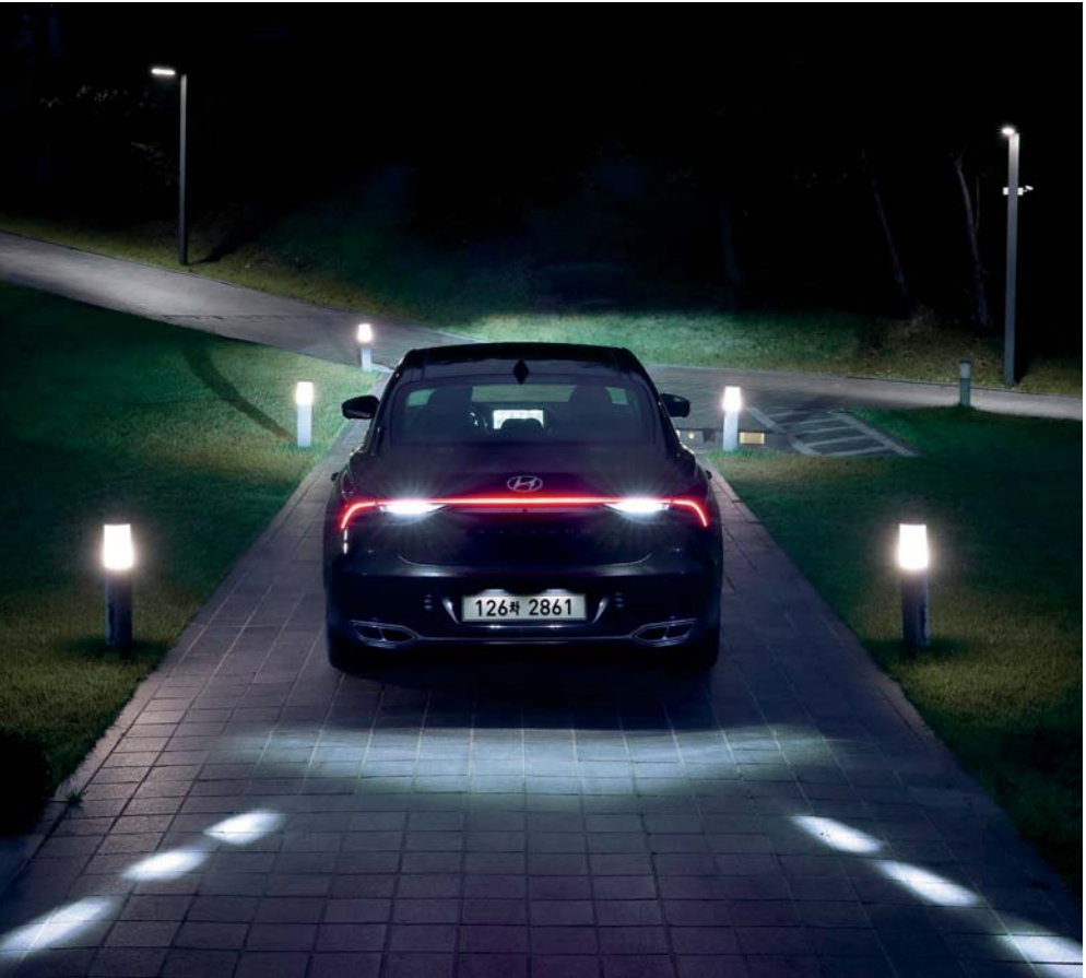
Back up guide lights When the car is backing up, “guide lights” are projected onto the road behind the car to clearly show the driver's intention to back the car up to prevent accidents involving nearby vehicles or pedestrians.
