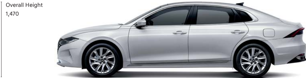
Overall Height 1,470 Wheel Base 2,885 Overall Length 4,990
