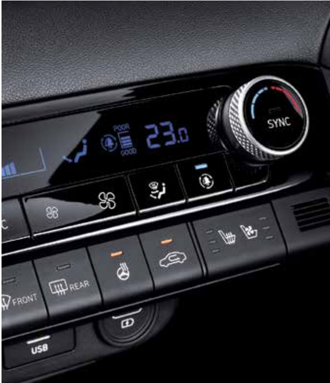
Air Purifying System AVANTE's air purification system uses a fine dust sensor to monitor the vehicle's interior air quality, activating an automatic air purifier when needed to ensure a more pleasant atmosphere.
