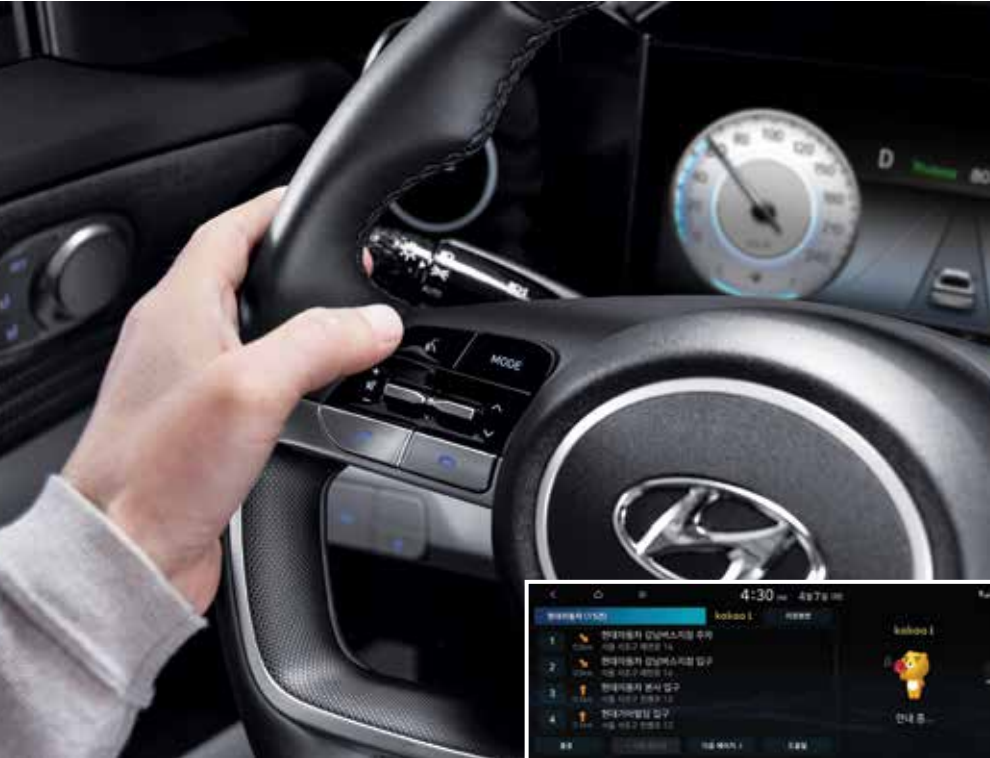
Voice Recognition Vehicle Control Adjust the climate control system and heated seats and access a variety of useful information with your voice—simply press the voice recognition button on the steering wheel and say what you want. * Use of Kakao i Voice Secretary requires an active Blue Link membership.
