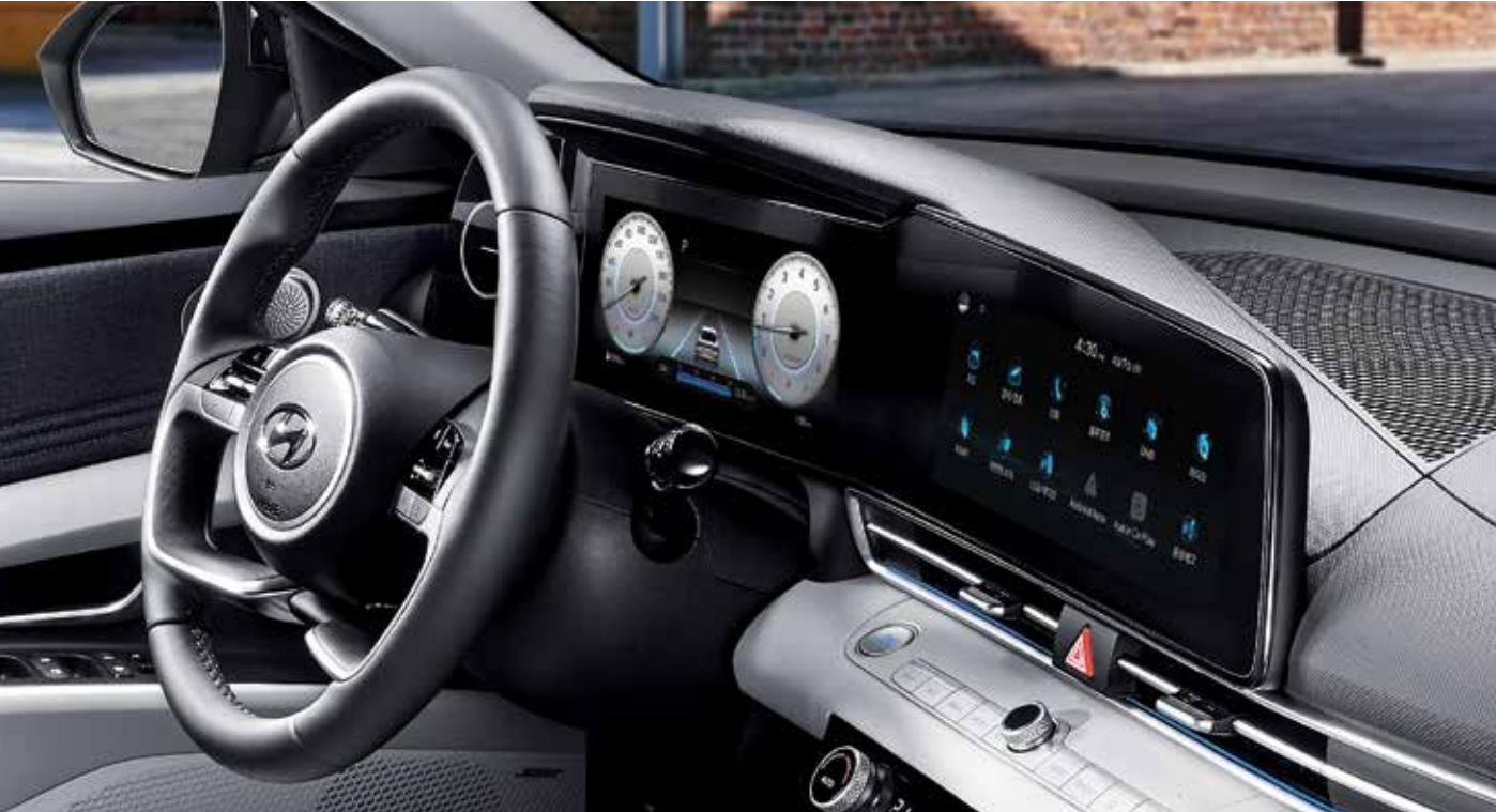
Panoramic Display A full color cluster display and navigation screen (both 10.25") deliver a seamless integrated panoramic view, tilted 10 degrees toward the driver for easier control and a high-tech feel.
