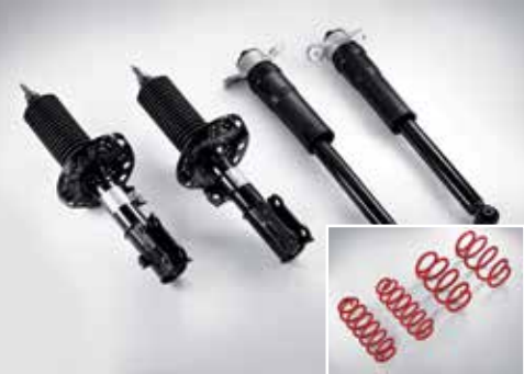
Monotube Shock Absorbers & Red Lowering Springs
