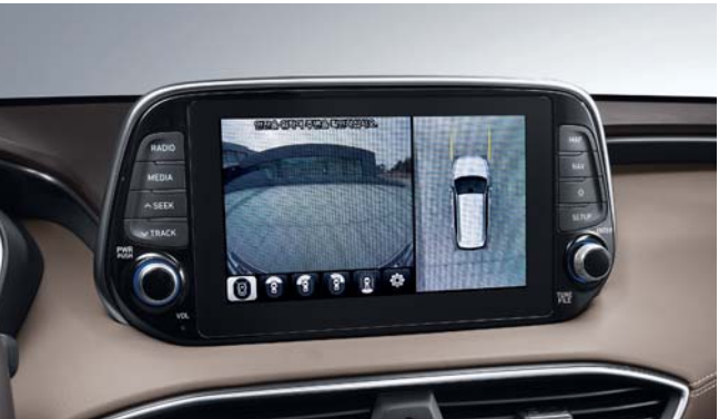
Rear view monitor (DRM) In case your view behind the vehicle via the rearview mirror is blocked by passengers in the rear seat or objects in the cargo area, this monitor shows real-time video footage of the space behind the vehicle.
