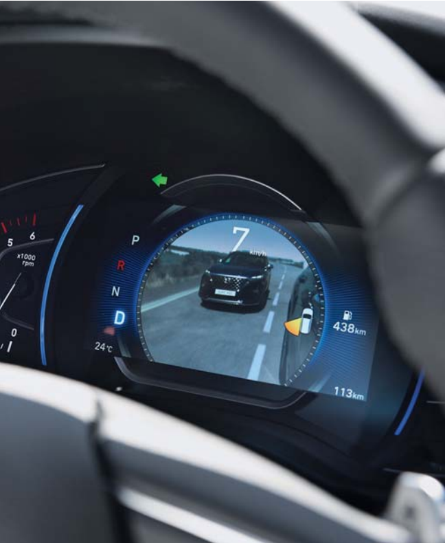
Blind-spot View Monitor Activating the turn signal causes video showing rear lateral views (right and left) to appear on the cluster screen through cameras attached to the base of the outside mirrors. In the event the driver's rear lateral view is obstructed (driving in the rain, blind spot, etc.), this function offers a clear and wide view to ensure safer driving.
