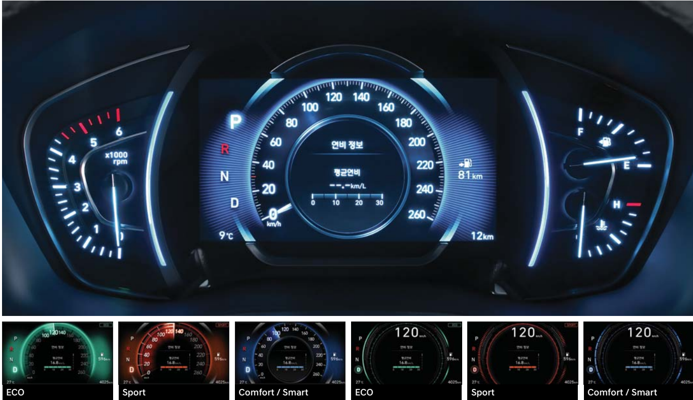
7-inch color LCD virtual cluster The dashboard changes color depending on the driving mode (Comfort / Smart, ECO, and Sport), adding a touch more fun to the driving experience. The wide and highly legible 7-inch LCD cluster display offers clear images that provide the driver with a range of information on the vehicle.
