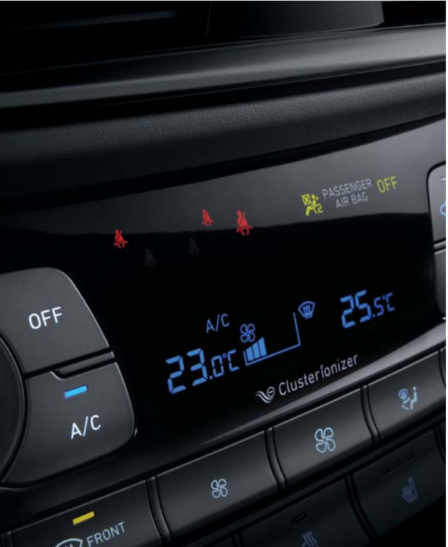
Whole seat belt reminder This function detects whether passengers in both the front and back rows are wearing seat belts. If one or more passengers are not wearing a seat belt, a warning light or sound is activated.
