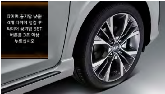
Tire Pressure Monitoring System Changes in the tires' radius and vibration are tracked to alert the driver when air pressure falls below preset conditions.
