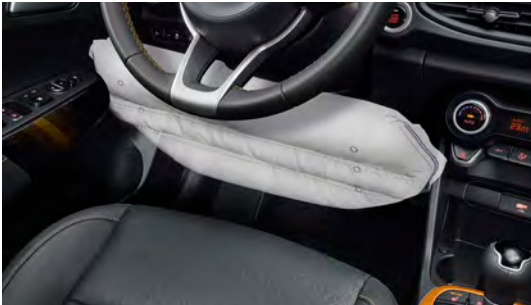
7-airbag system* 7-airbag system includes a driver's airbag, front airbag, side and curtain airbags, and a knee airbag that protects the driver's knees. Driver's knee airbag*
