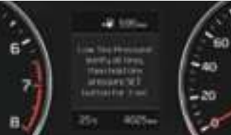
Indirect TPMS Using the ABS system's wheel speed sensors, indirect TPMS detects air loss in tires through differences in relative wheel speeds.
