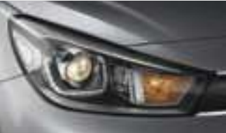
Bi-projection headlamps Bi-projection headlamps offer increased illumination, enabling you to better detect obstacles and the road ahead.
