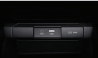
Auxiliary and USB connections Flash drives and other compatible audio devices can be connected via 3.5 mm (analog) and USB ports.
