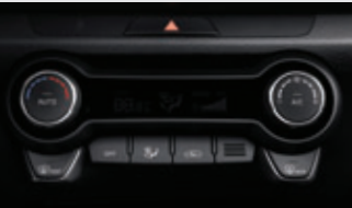
Full Auto Temperature Control (FATC) FATC lets you set a desired temperature for a comfortable ride in any weather condition.
