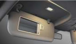
Sunvisor illumination lamps Bulb lamp over the vanity mirror on the driver-side sunvisor lights up to help you see yourself better in the mirror.
