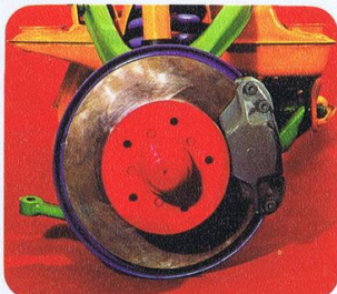
All Mercedes-Benz models have dual-circuit servo-assisted disc brakes on all four wheels.
