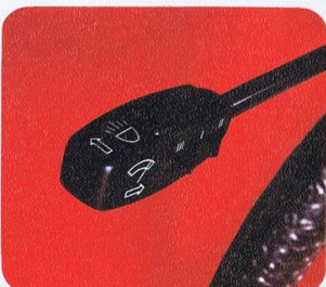
The combination switch on the steering column operates headlight flasher, high beam headlights, indicators, fingertip contact for changing lanes, windshield wipers with two speeds and intermittent control.
