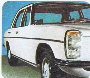
The bodywork has all-round protection. Wide rubber strips in the bumpers at the front and rear, and rubber inserts in the chrome strips along the sides.
