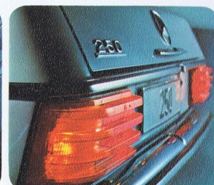
The ridged profile of the rear light unit helps prevent dust and dirt clinging to the surface.
