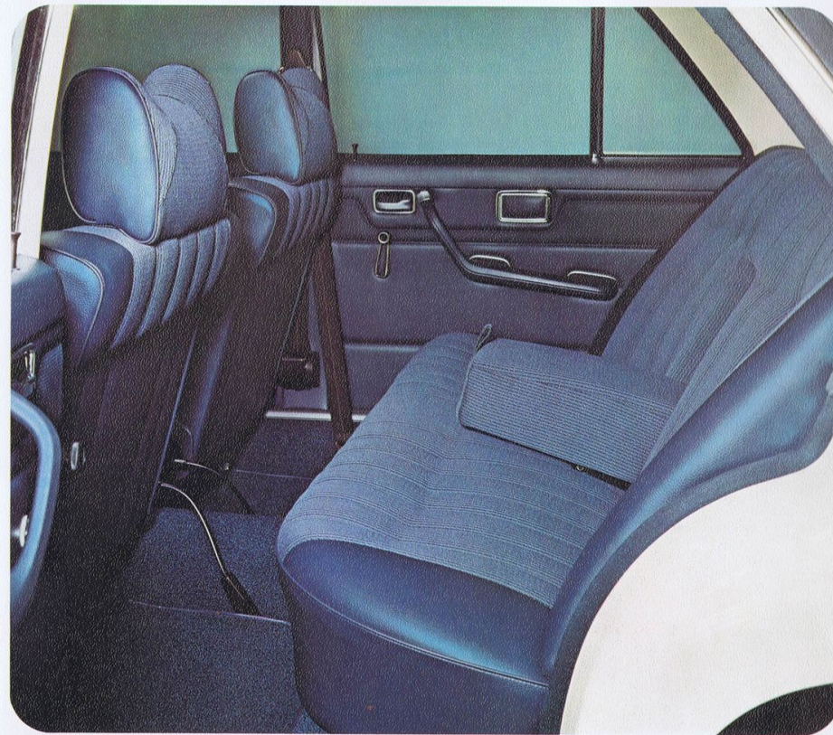
Between the rear seat with its folding centre armrest – seat depth 19.7 in., overall width 58.5 in. – and the front seats, passengers in the back have ample legroom. Space is not the only criterion for comfort. Anatomically-contoured seats, the result of exhaustive physiological research, also contribute.
