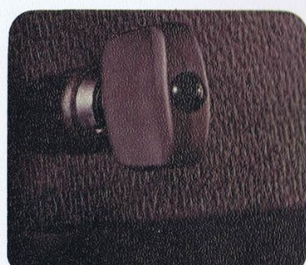
All switches, levers and handles are flexible or flush-mounted. One switch controls headlights, parking lights, foglamps, rear foglight and side lights.
