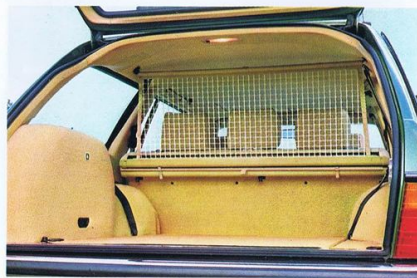
The retractable net serves as a partition between passengers and the load.
