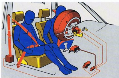
Electronically-controlled restraint system with airbag and belt-tensioner.
