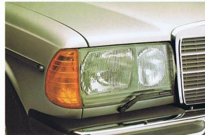
Halogen headlamp unit with integral foglamp and wrap-around directional indicator.
