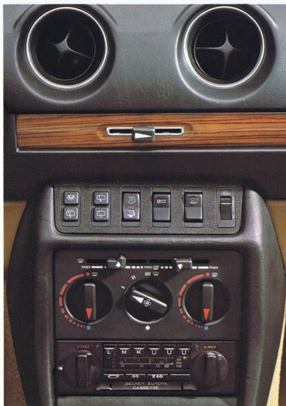
Continuous, draught-free flow of warm or cold air with three-stage booster fan for windscreen, side windows and front and rear footwells.
