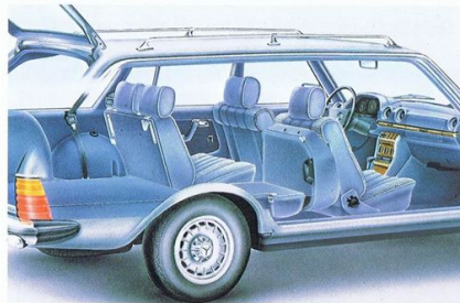
Room for four people; part of rear bench seat folded away to increase load compartment length to 1.78 metres.
