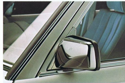
Rear-view mirror, adjustable from inside the car, in an aerodynamically-shaped bracket.
