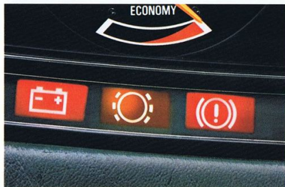
The brake pad wear indicator reminds you in good time that the brake pads need to be replaced.
