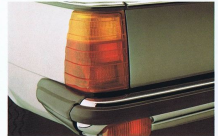
Large, rear-light units with ribbed profile, so they get less dirty.
