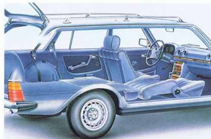
Room for one person. For particularly long items, up to about three metres (nearly 10 ft), the front passenger seatback can be fully reclined.
