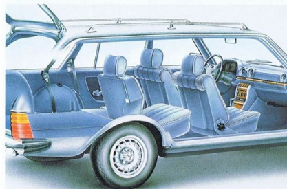
Room for three people; two thirds of the divided rear bench seat (optional extra) folded away, rear seatback removed.
