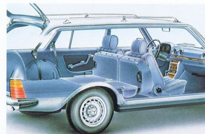
Room for two people and a load space that is 1.78 metres long and up to 1.48 metres wide, with the rear bench seat folded away.
