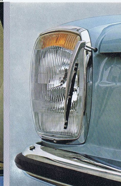
Headlight cleaning equipment
