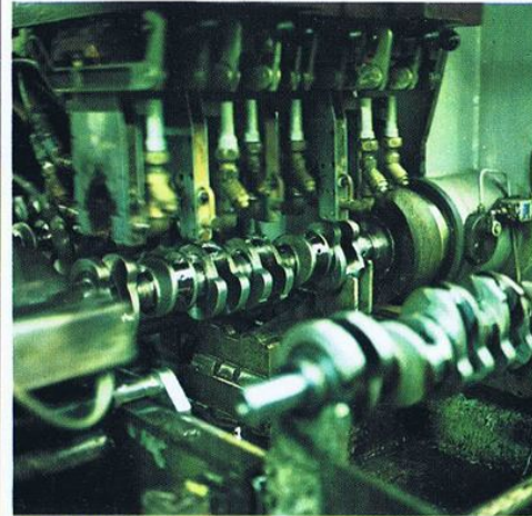
Inductive hardening means that the important points receive particular attention without the surface structure being affected. Nothing is left to chance.
