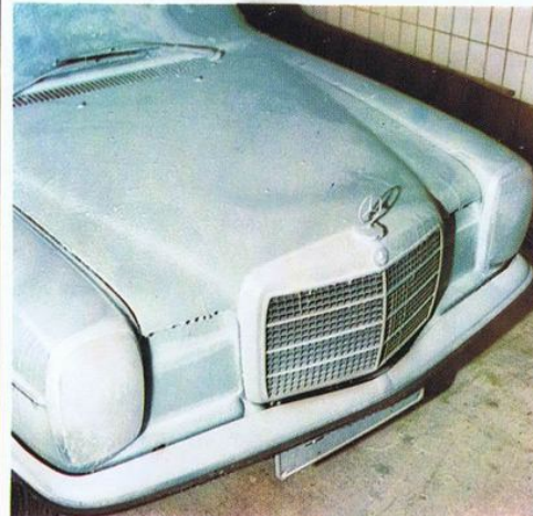
Part of the development programme. A car is put into the cold room, where the temperature is -25^{\circ}\text{C} . To pass the test the engine must start in 10 seconds.
