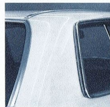
Ventilating slots on the side of the rear window
