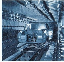
Cooling after the paint annealing process
