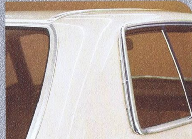
Ventilating slots on the side of the rear window
