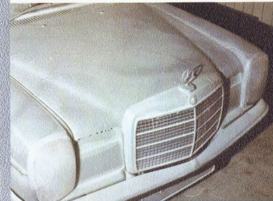
Starting test in the cold chamber
