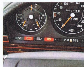
Warning lights, with symbols, for indicators, high-beam headlights, fuel reserve, battery and brakes.
