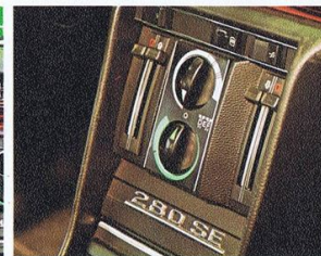
Located on the centre console, heating and ventilation levers, ashtray and optional special equipment (radio and air-conditioning unit).
