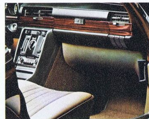
The progressively-yielding instrument panel was developed in decades of research. The knee protection below it, is new.
