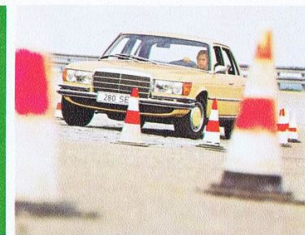
The front wheels tilt when the steering wheel is turned and therefore brace themselves against the road, thus providing high cornering speeds.
