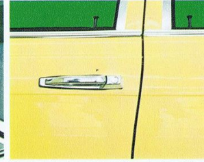
Counterbalanced safety lock with rounded, pull-type, door handle. It will not burst open or jam under impact.
