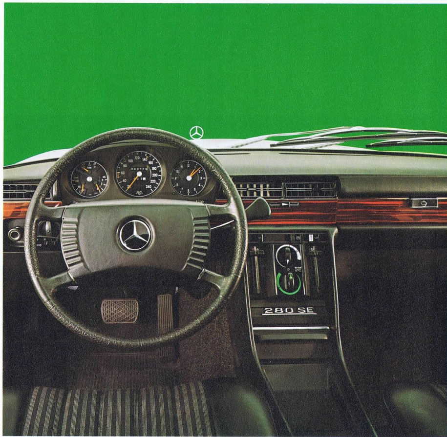
The 280 S and 280 SE models have floor gear shift as standard. Both cars can, however, be supplied with column gear shift, when fitted with Mercedes-Benz automatic transmission.
