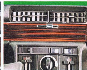
A total of 11 adjustable air vents. In the middle of the instrument panel, a large fresh-air vent infinitely adjustable to all angles.
