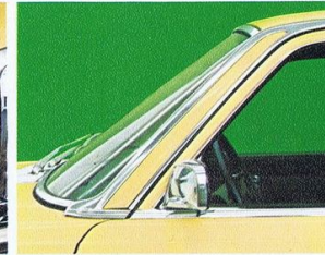
Side windows remain free from dirt, due to newly designed, extra sturdy, roof pillars. Rainwater is directed away from the windows.
