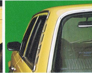
Draught-free, continuous ventilation by means of extractor slots in the rear roof pillars. Complete change of air three times a minute, even when the windows are closed.
