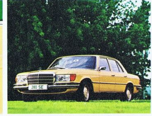
Despite its 11.5 cm longer wheelbase (compared with their predecessors) both cars have a turning circle diameter of only 11.4 m.
