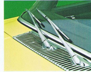
Two-speed windscreen wipers with intermittent control. Correctly located in the air flow on the screen, there is no danger of "lifting" at high speed.
