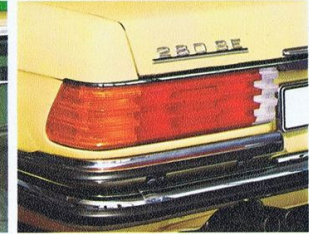
The rearlight unit repels dirt, because of its ridged surface, developed in the wind tunnel.
