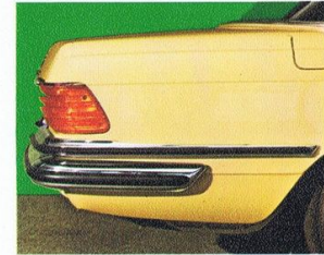
The bodywork has all-round protection. Wide rubber strips in the bumpers at the front and rear, and rubber inserts in the chrome strips along the sides.
