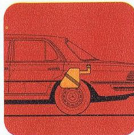
Safety fuel tank
