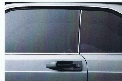
Door-handle set in dirt-deflecting panel. There is a rain-water outlet in the barrel of the lock.
