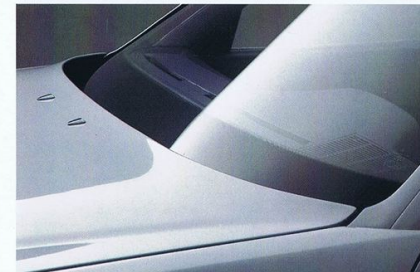
Recessed windshield wipers, with overload protection.
