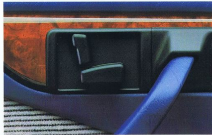
With this switch, the front seats can be adjusted, electrically, to eight different positions.
