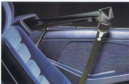
Belt-guides automatically move the seat-belts towards the driver and front-seat passenger.
