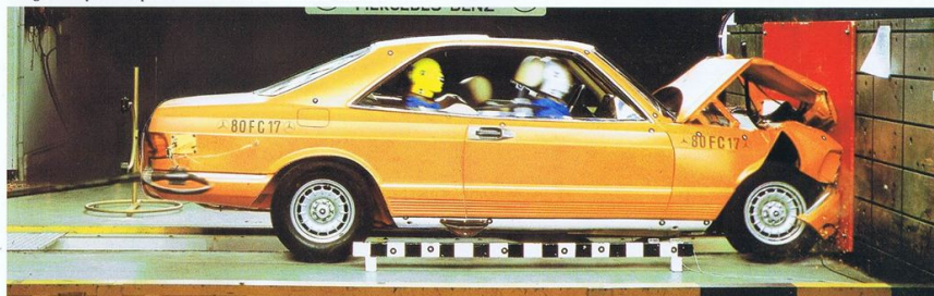
The longer crumple zone has progressive degrees of rigidity, giving the greatest possible protection in head-on and rear-end collisions.
