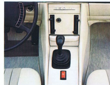
Floor shift with logically arranged gearshift pattern. For reasons of safety the gear lever knob was provided with foam padding.
