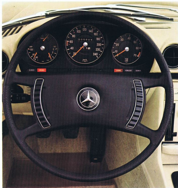
The four-spoke safety steering wheel. The padded boss, spikes and rim form one foam-padded unit.
