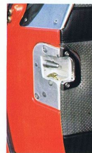
The strong pin of the safety lock. The door handles have no projecting knob. The doors are opened by pulling the door handle.
