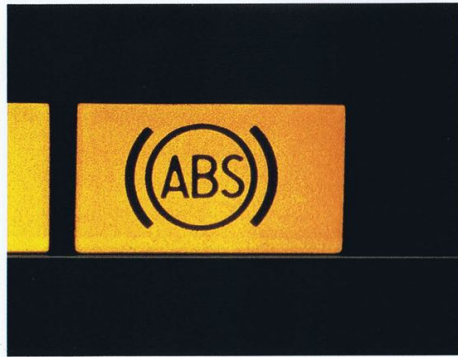
The anti-lock brake system (ABS). Even with the brakes full on, the car can still be steered.
