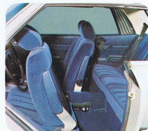
The front seat back rests tip forward. They can be fixed by a vacuum locking device and can only be released by pressing a knob.
