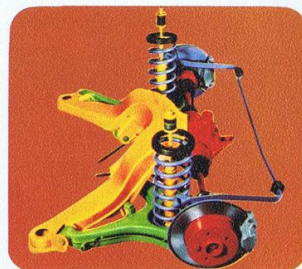
The Mercedes-Benz diagonal swing axle ensures perfect roadholding in any situation.
