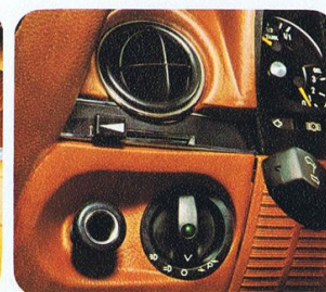
All knobs, switches and levers are flexible or flush-mounted. One central switch for headlights, parking lights, foglamps, rear fog light and side lights.
