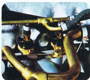
Two of the eight injection elements of the V8 engine.
