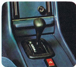
The automatic 3 speed transmission with torque convertor and floor shift are standard fittings on the 450 SLC.
