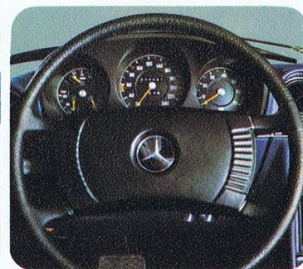
Mercedes-Benz safety steering with large padded boss on the steering wheel, impact absorber under the padded boss; telescopic steering column; steering box located well
