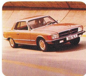
The SLC models are driven by a powerful V8 engine with electronically controlled fuel injection.
