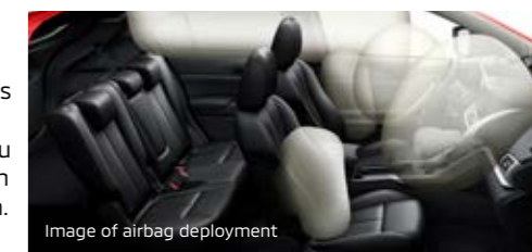
Image of airbag deployment (Optional side airbags and curtain airbags for RHD. Optional side airbags, curtain airbags and driver's knee airbag for LHD.)
