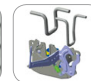
Hood safety mechanism with double striker
