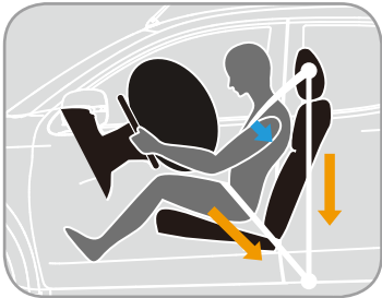
Double pretensioner (Driver's seat)
