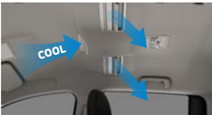
Air circulator for rear passengers NEW An air circulator installed in the ceiling ensures that passengers in the rear seats can relax at an ideal temperature. The circulator efficiently moves air through the cabin space, and wind direction and power are adjustable so that everyone can enjoy a refreshing breeze.
